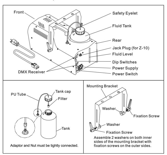
**Note:** A fluid level sensor is installed on the unit. The machine will stop to fog if the fluid is lower than usable level.
